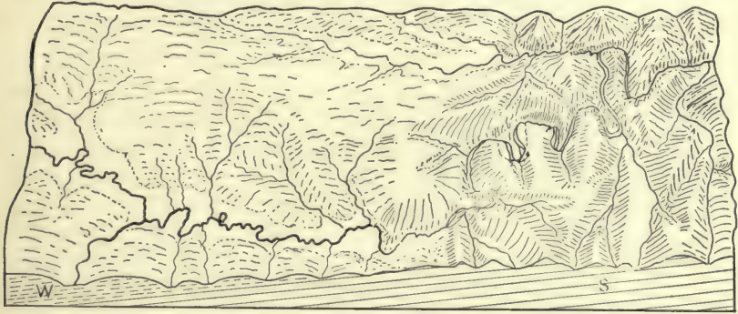
FIG. 156.—The upper Osage valley is underlain by weak rocks ( W ) and is eroded to an old surface. The lower valley underlain by strong rocks ( S ) is eroded only to a mature stage. The river flows from left to right.
